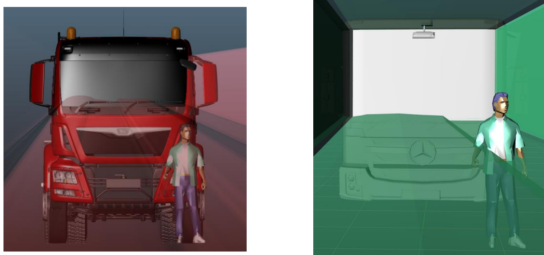
Figure 3.2. Illustration of moving off collision scenario, pedestrians not visible (left) and partially visible (right)
