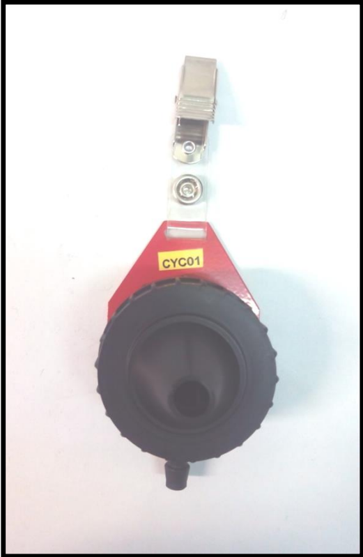
Figure 10. Cyclone Inhalable Sampler to monitor PM 2.5.
