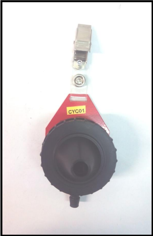
Figure 10: Cyclone Inhalable Sampler to monitor PM 2.5.
