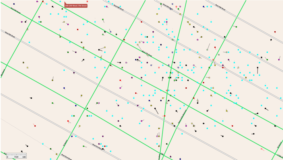
Figure 36: Cartographic Display of NDL Remotely Sensed GPS Vehicle Position-Time Data (showing urban canyon scattering that occurs around midtown Manhattan)
