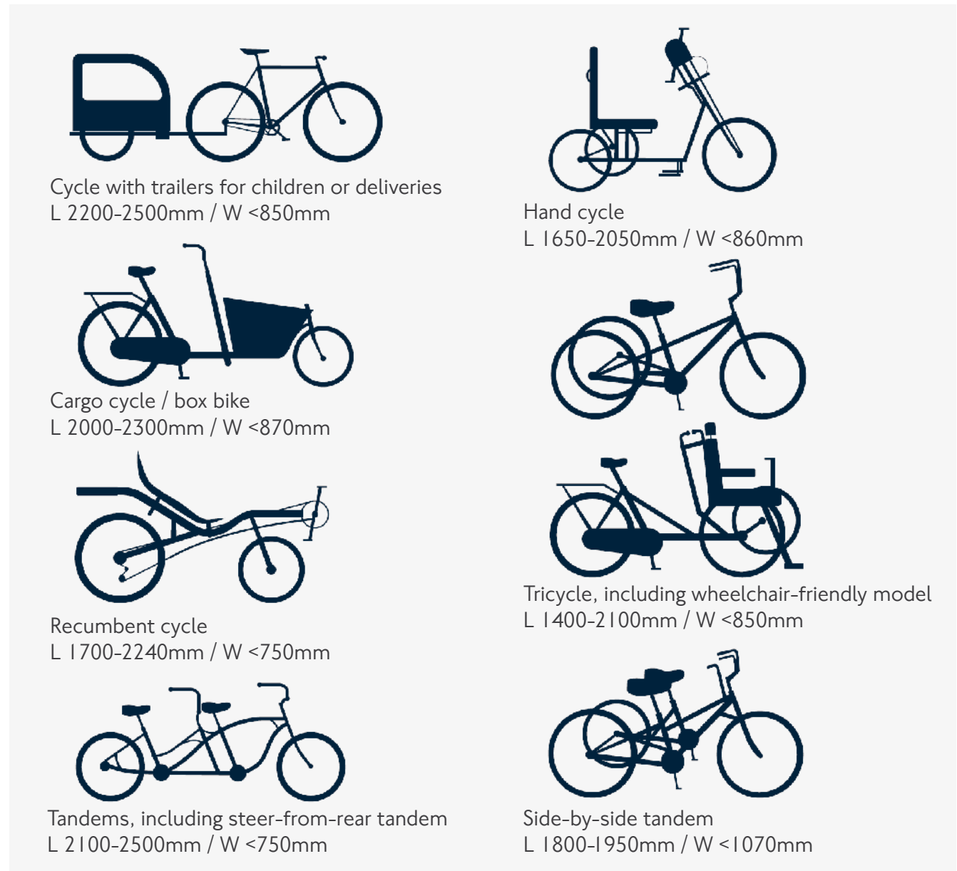
Figure 3.4 Indicative dimensions of typical ‘non-standard’ cycles
