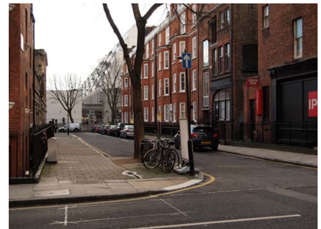
Footway build-out incorporating cycle parking
