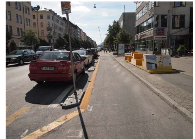
Trial measures on Gotgaten, Stockholm: car and cycle parking moved out into the carriageway to create more protected space for cycling. The existing, stepped cycle track has been used for temporary seating
