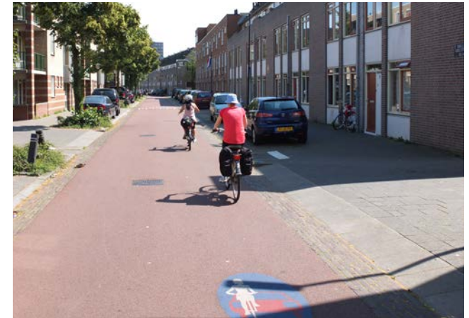
Surface marking shows cycle street status
