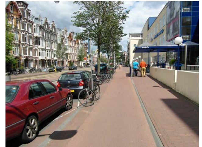
Separation using car parking in Newham (left) and parking and street furniture in Amsterdam (right)
