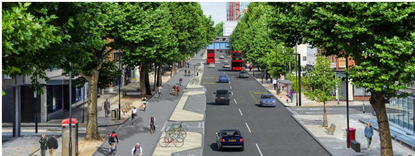
Visualisation of Cycle Superhighway scheme for Blackfriars Road, where side roads and active uses are predominantly on the east side and a two-way track is therefore proposed for the west side.
