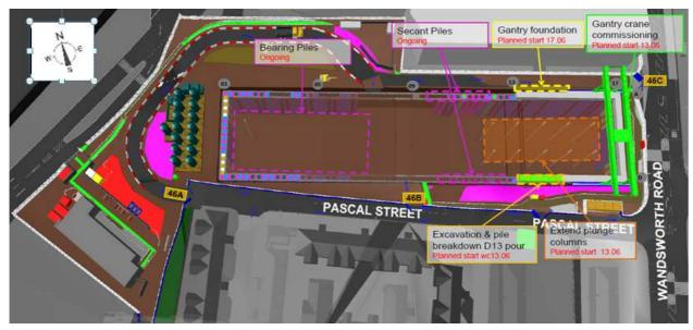
We will resume the works associated with the capping beam construction following the completion of the piling works. These works will mainly progress from east to west.
