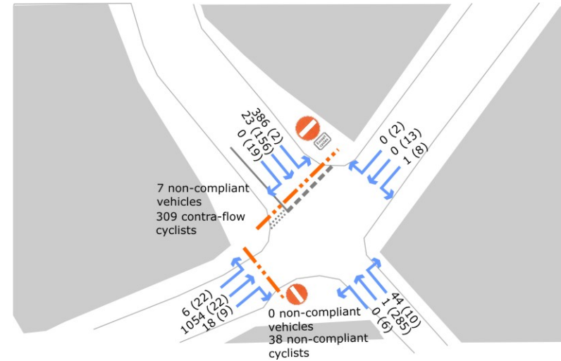
Stockwell Avenue/Bellefields Road Junction - After
