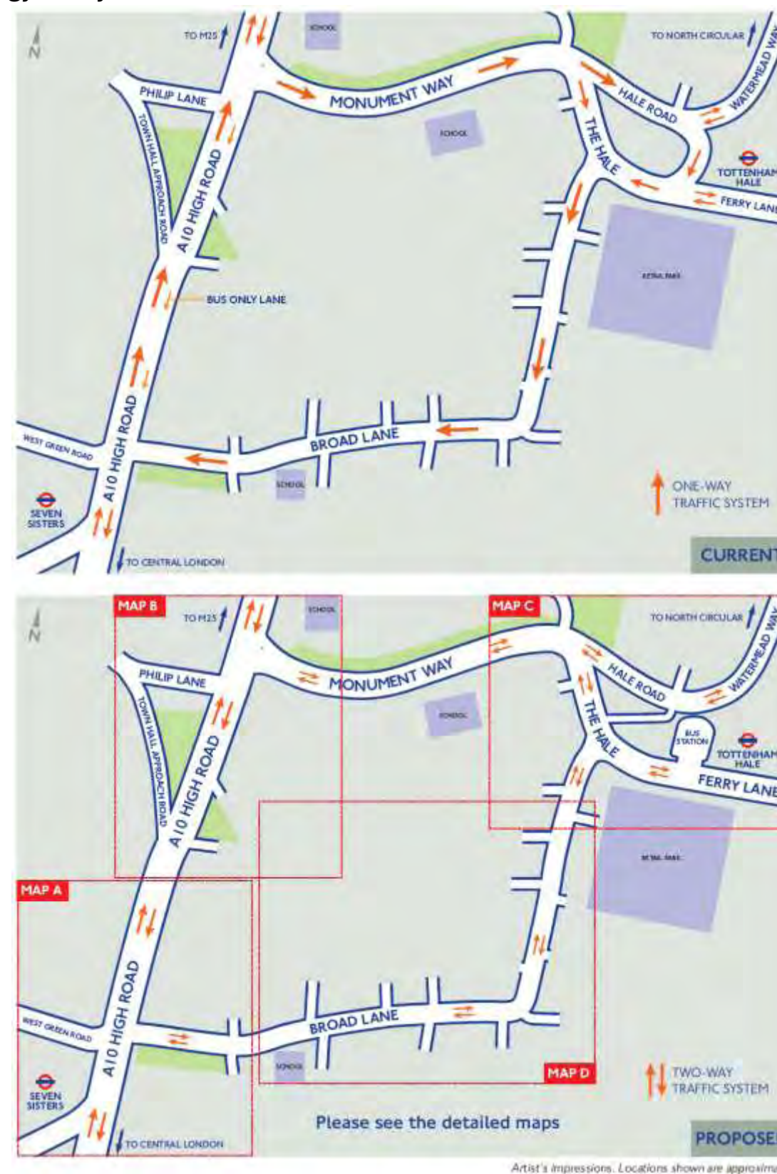
Figure 3.3: Maps showing current and proposed lay out for Tottenham Hale gyratory
