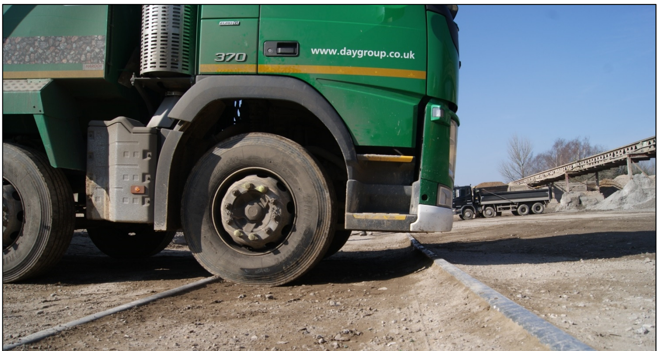
Figure 3-6 Vehicle approach angle sufficient to clear railhead
