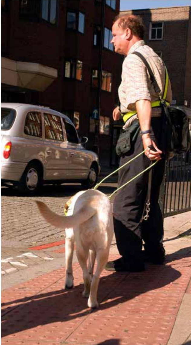
Figure 123: Tactile paving is used to communicate important information to the visually impaired
