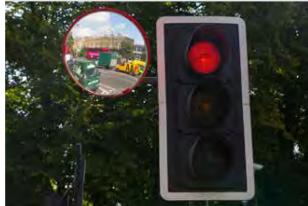
Figure 159: Trixi mirrors are used by motorists at junctions to detect cyclists in their blind spot
