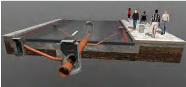
Figure 274: A typical highway drainage system. There are features visible on the surface, such as covers and gratings as well as those buried and out of sight such as pipes and chambers
