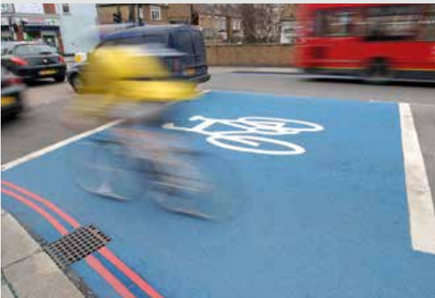
Figure 109: An advanced stop line coloured in sky blue on a Cycle Superhighway
