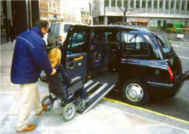
Figure 31 I: Taxi set down and pick up areas should have a minimum kerb height of 140mm
