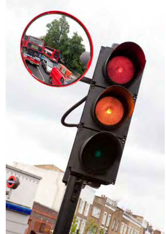
Figure 288: Trixi mirrors are used by motorists to see their blind spots at junctions
