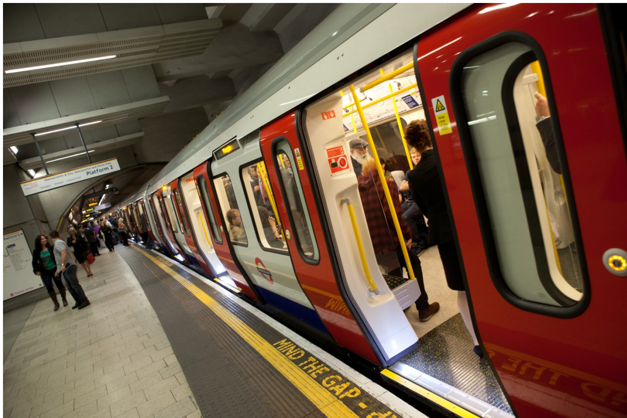
New air-conditioned, walk-through trains on the sub-surface railway
